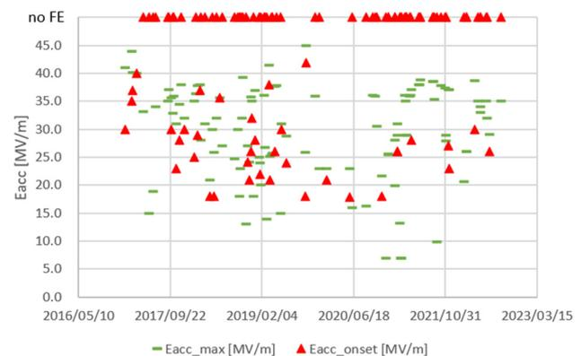
Figure 4: Maximum accelerating gradient (green bars) and onset gradient (red triangles) over time for VTs of single cell cavities.
