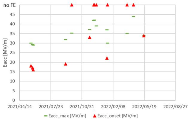
Figure 5: Maximum accelerating gradient (green bars) and onset gradient (red triangles) over time for VTs of 3-cell cavities.
