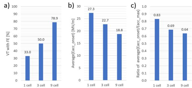
Figure 7: Comparison of single cell, 3-cell, and 9-cell cavity tests: a) percent of tests showing FE, b) average onset gradient, c) ratio between onset gradient and maximal accelerating gradient.
