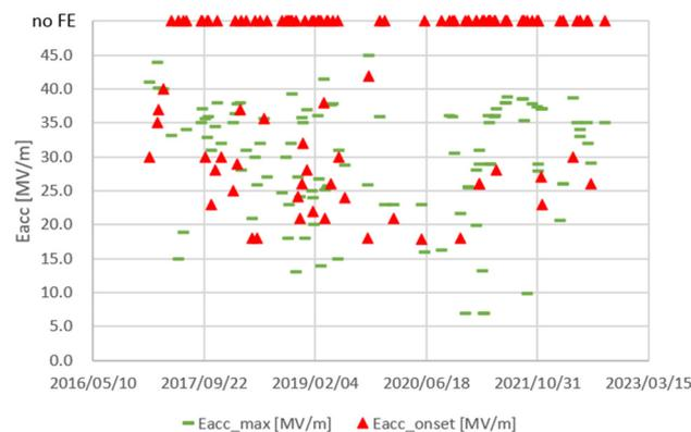
Figure 4: Maximum accelerating gradient (green bars) and onset gradient (red triangles) over time for VTs of single cell cavities.
