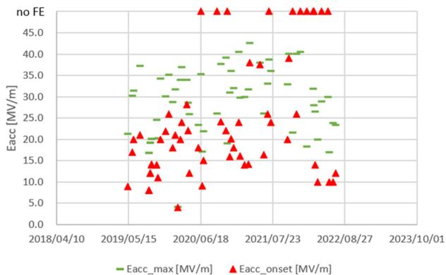
Figure 6: Maximum accelerating gradient (green bars) and onset gradient (red triangles) over time for VTs of 3-cell cavities.
