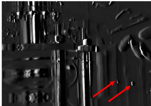
Figure 3: Scattered light of particulates passing through fanned out laser beam.
