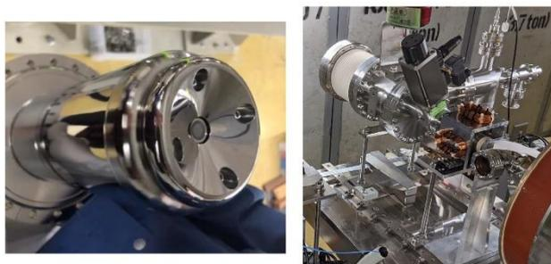
Figure 2: Pictures of the cathode part (Left) and the thermionic electron gun (Right).
