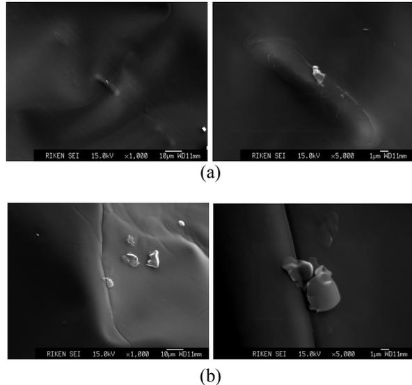
Figure 3: SEM images of the GTF disk surface. (a) no-irradiated part and (b) beam-irradiated part.
