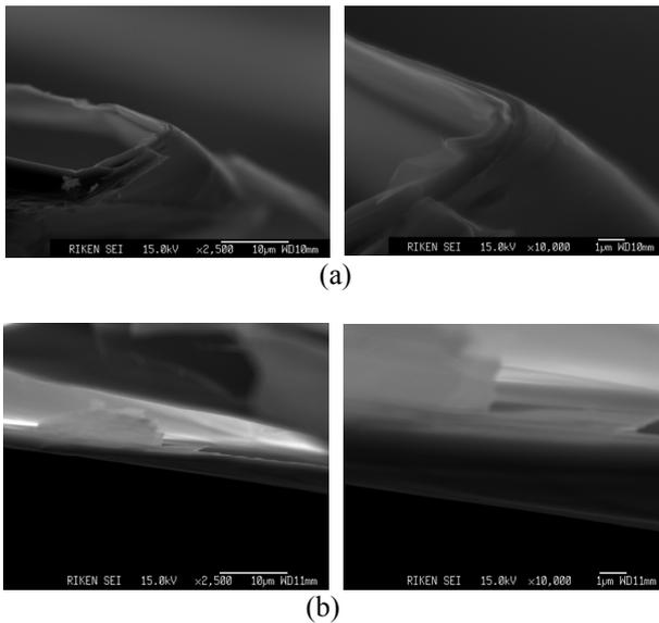
Figure 4: SEM images of the GTF disk cross-section: (a) no-irradiated part and (b) beam-irradiated part.
