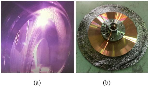
Figure 1: (a) GTF disk during U beam irradiation. The irradiated spot was brilliant. (b) The GTF disk after the beam operation.
