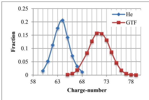
Figure 2: Charge distributions of the U beam at 10.75 MeV/u after passing through the GTF disk (solid squares) and the He gas stripper (diamonds).
