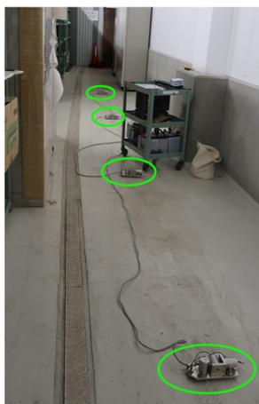
Figure 16: Sensors for wave velocity measurement.
