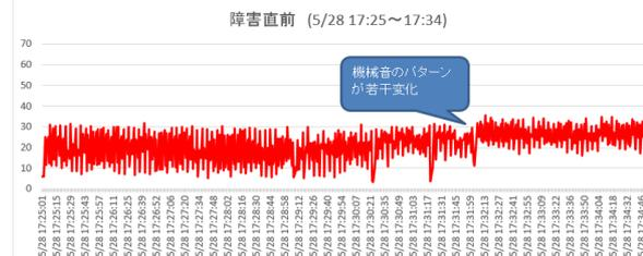
Figure 12: Anomaly Score just before failure.
