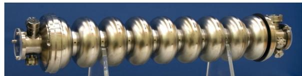
Figure 2: 1.3 GHz SRF cavity (length 1.3 m).
