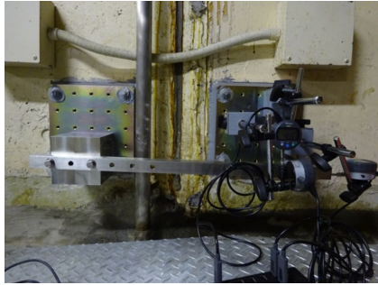
Figure 3: Setting of dial gauges.
