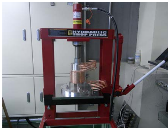
Figure 7: The FC head was pressed by a hand press machine.
