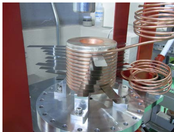
Figure 8: Sim plates of 0.2mm or 0.3mm thickness were inserted into the slits to expand their gap.
