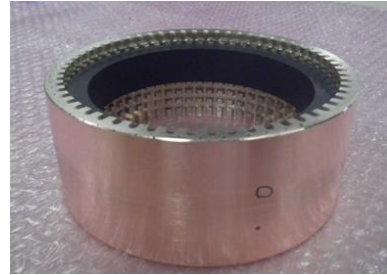
Figure 3: An AlN cylinder brazed to a copper cylinder.
