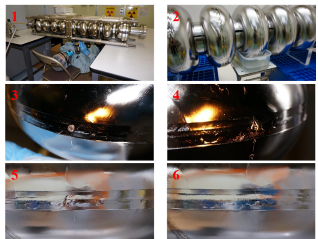
Figure 5: Repairing steps of the hole. Each numbers correspond to ones in context.
