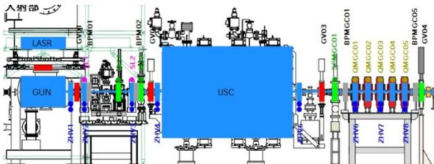
Figure 3: Layout cERL of injector line.
