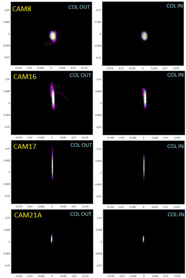
Figure 5: Simulated beam halo profiles.
