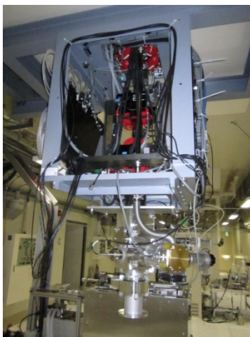
Figure 8: Picture of new Irradiation port for RI production.
