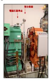
Figure 4: Measure the shape of girder surface and the heights of magnets.
