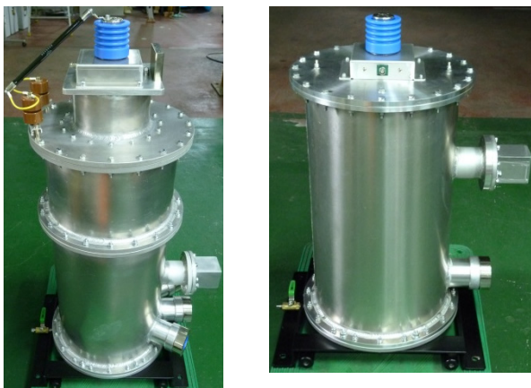
Figure 4: photographs of a pulse compressor for a horizontal magnet (left) and a pulse transformer for a vertical magnet (right).
