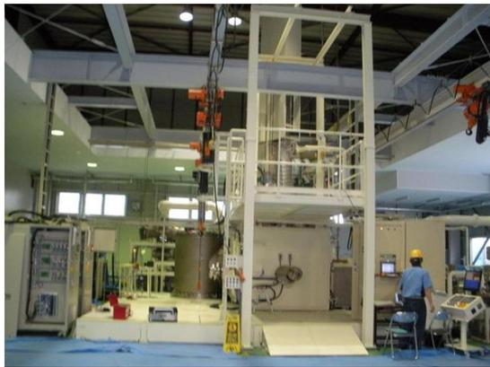
Figure 1: Appearance of 600kW EB furnace.
