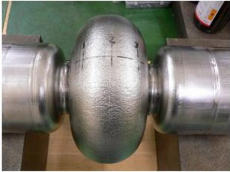
Figure 10: Single cell Nb seamless cavity.
