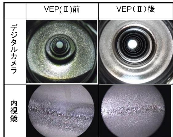
Figure 8: Inner surface of cavity before and after VEP(II).
