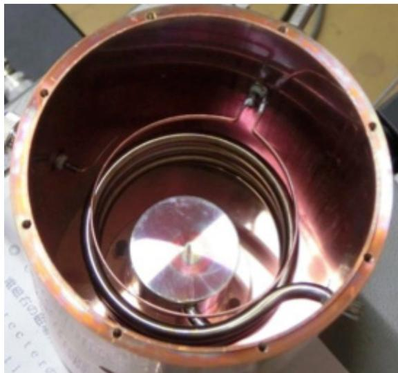
Figure 4: Fabricated RF resonator (seen from upstream).
