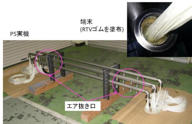
Figure 7: P5 signal cable ducts
