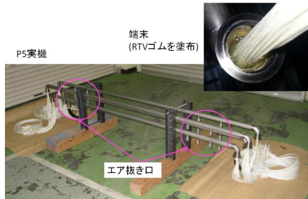
Figure 7: P5 signal cable ducts
