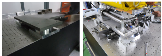
Figure 10: LAPP-support and side blocks.
