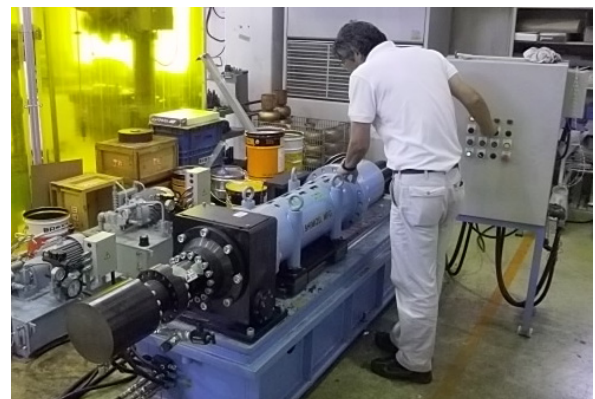
Figure 3: Hydroforming machine (Final hydraulic pressure: 25 MPa).
