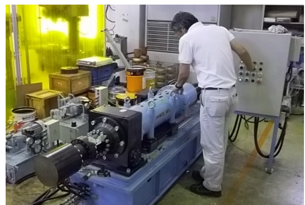
Figure 3: Hydroforming machine (Final hydraulic pressure: 25 MPa).
