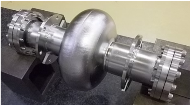
Figure 6: Finish to 1-cell cavity.
