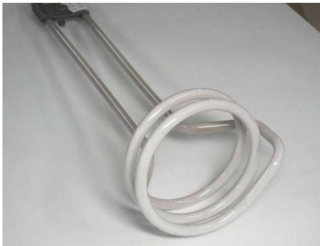
Figure 3: RF-Antenna developed in SNS.
