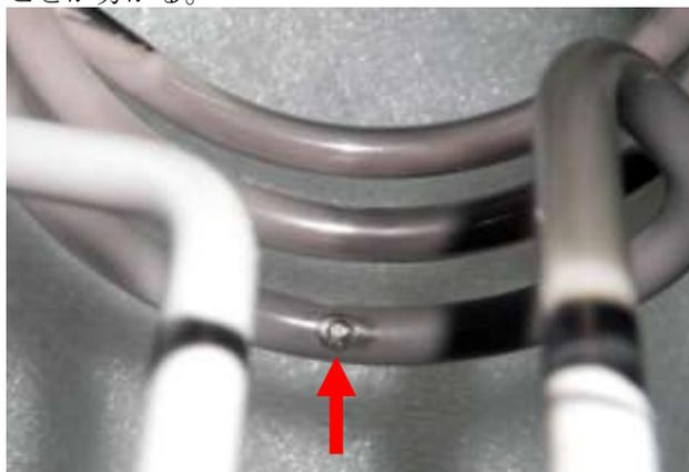
Figure 8: Photograph of damaged the RF-antenna.
