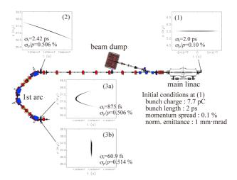
Figure 3: Change of time-momentum (t, p) distribution of the electron bunch from before the main linac to after the  $1^{st}$  arc section in the bunch compression process. The numbers on the distribution plots mean their temporal order. (3a) and (3b) correspond to two cases of SX1-4 OFF and SX2&4 ON listed in Table 1. The bunch length and momentum spread are also shown on each plot. In the simulation, the bunch length is minimized at the exit of the  $1^{st}$  arc section.
