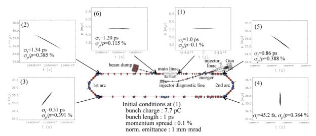
Figure 4: Change of time-momentum (t, p) distribution of the electron bunch along the cERL when SX2 and SX4 are used. The numbers on the distribution plots mean their temporal order. The bunch length and momentum spread are also shown on each plot. In the simulation, the bunch length is minimized at the entrance of the  $2^{nd}$  arc section (4) and the momentum spread at the entrance of the dump line (6).
