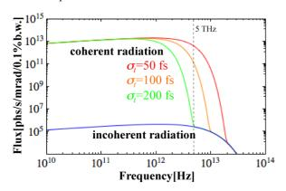
Figure 1: CSR spectra of the 20 MeV cERL for three different bunch lengths of 50, 100 and 200 fs, at the bunch charge of 7.7 pC and the bunch repetition frequency of 130 kHz.
