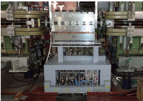
Figure 10: Damper cavity in CERN PS.
