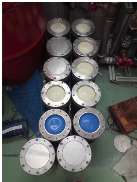
Figure 4: Photograph of damaged capacitances used in a PFN of a klystron modulator. The explosion proof valves of eight capacitances are already opened. Two blue colored capacitances were transported from Waseda University.
