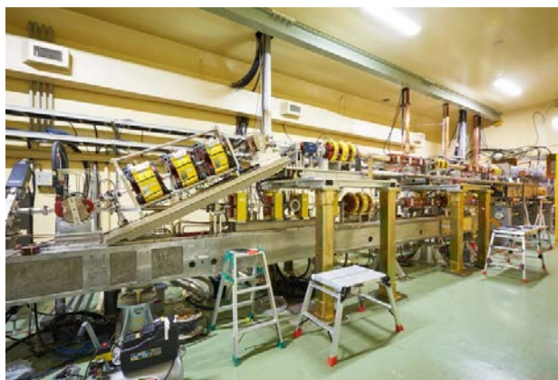
Figure 6: Thermal electron gun and RF electron gun.
