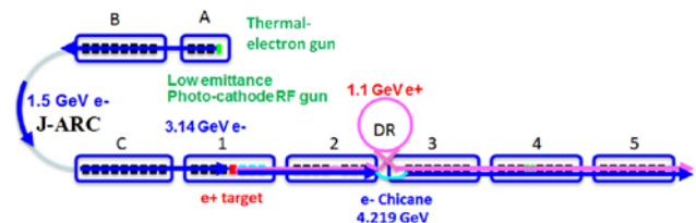
Figure 1: Layout of SuperKEKB injector linac.
