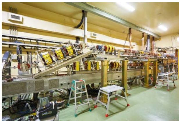
Figure 6: Thermal electron gun and RF electron gun.
