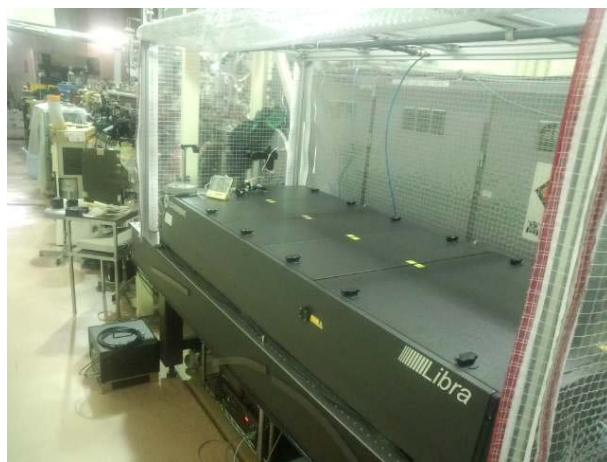
Figure 1: Er fiber laser for S-band photocathode RF-gun.
