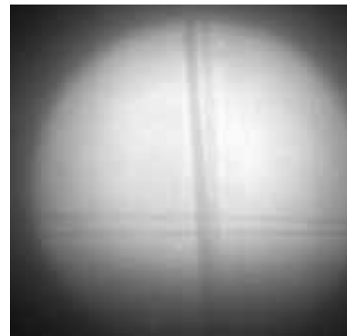
Figure 6: X-ray transmission image of bridge flange.
