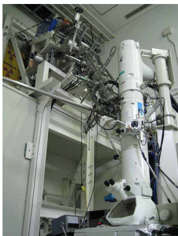
Figure 2: In-situ observation system with TEM at 1.7 MeV tandetron (RAPID).
