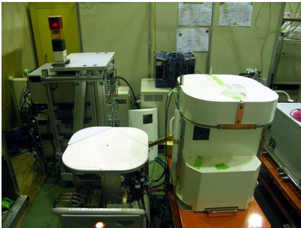
Figure 3: 950 keV X-ray source based on X-band Linac.
