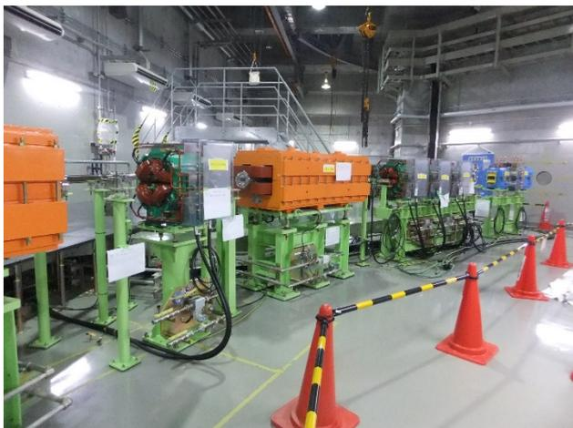
Figure 9: Installed magnets in the horizontal beam line for the room C.
