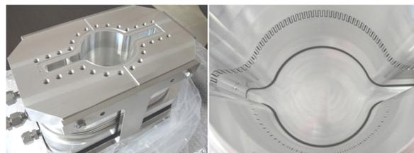
Figure 1: Typical structures of a beam pipe (up) and a bellows chamber for LER arc section (down).
