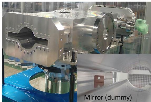
Figure 2: Vacuum chamber for a beam size monitor using the synchrotron radiation from a bending magnet. The mirror is located in an antechamber.
