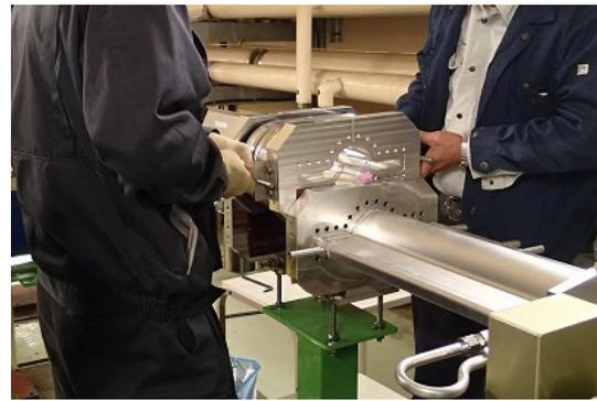
Figure 6: Connection of bellows chamber between beam pipes.
