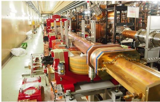
Figure 4: Copper beam pipes installed into wiggler magnets.
