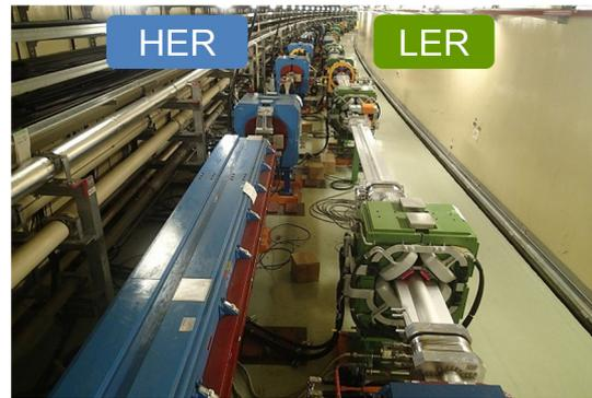
Figure 7: Installed HER and LER beam pipes in arc section.
