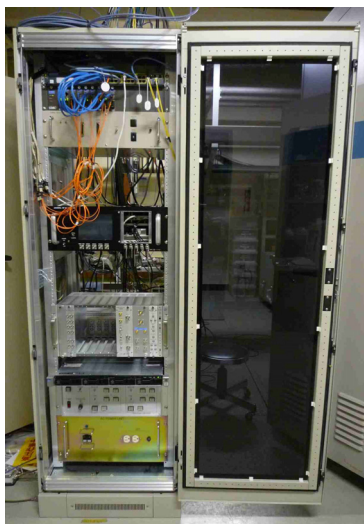
Figure 2: Layout of RF monitor rack.
