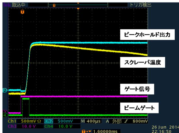
Figure 5: Waveform of temperature of scraper (400us/div).
