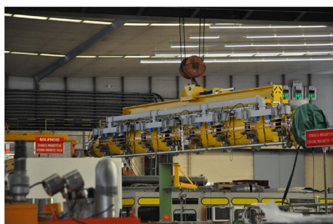
Figure 2: PDS assembled with cryomodule which is used in Euro-XFEL.
