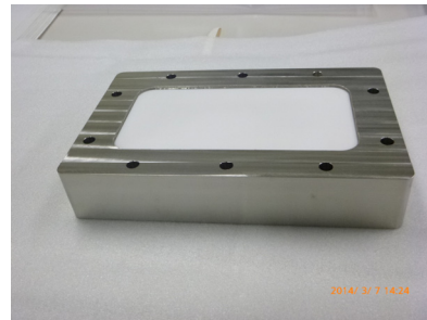
Figure 7: Rectangular waveguide window prototype.
