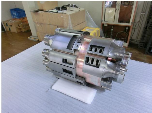
Figure 1: L-band RF gun before re-brazing. The outer surfaces of the ducts right above the welding parts are squarely cut to braze from inside
