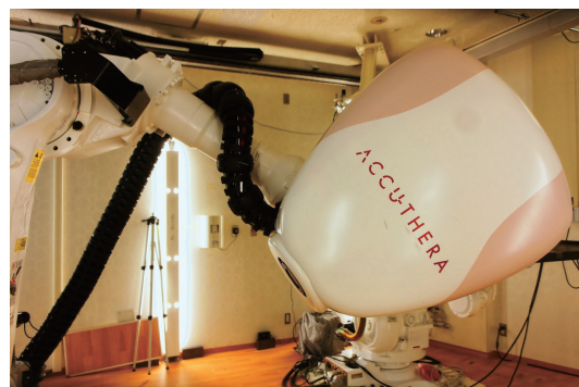
Figure 7: The X ray head containing the X-band 6 MeV accelerator.
