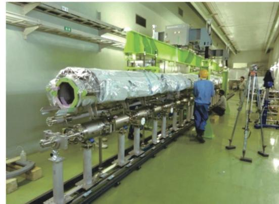
Figure 3: Picture of the ILC-type cryomodule CM-1 assembly in the tunnel, by using rail-system.
