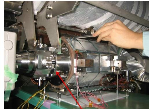
Figure 4: Conduction-cooled splittable quadrupole magnet was installed in the center of CM-1, together with BPM chamber.
