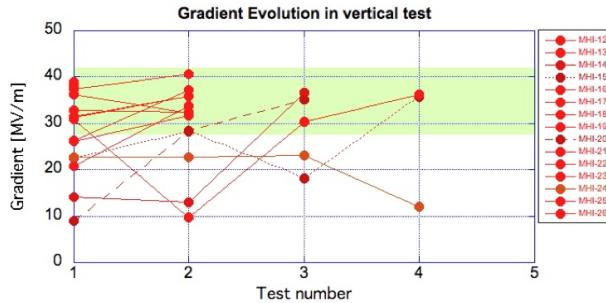
Figure 8: Transition of cavity gradient performance of each cavity.
