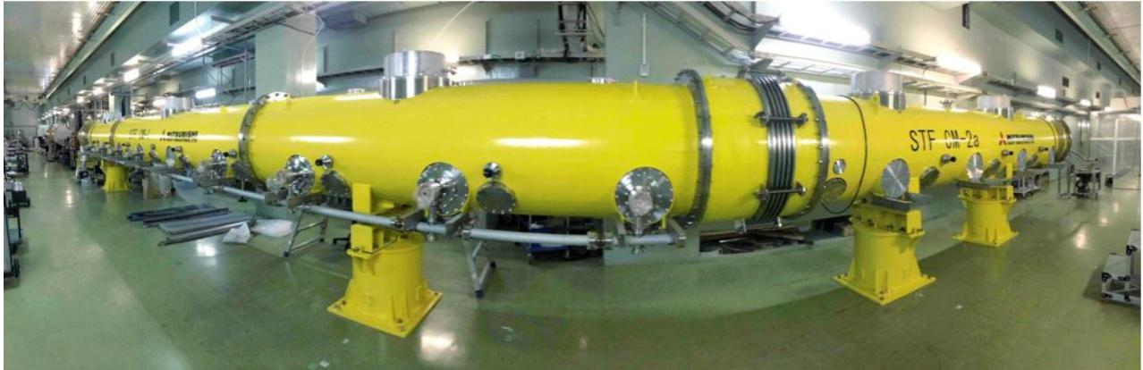
Figure 5: Picture of ILC-type cryomodule followed by the 6m cryomodule in the STF underground tunnel.
