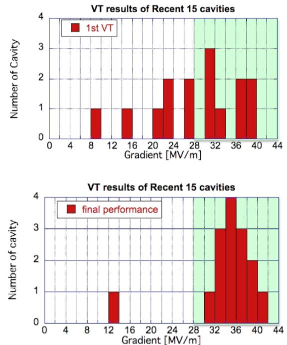
Figure 7: Cavity gradient performance of the cavity used in the STF accelerator.
