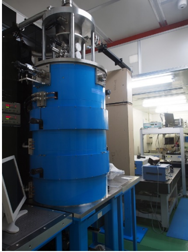
Figure 3: Photo of time-resolved relativistic-energy electron microscopy using RF gun
