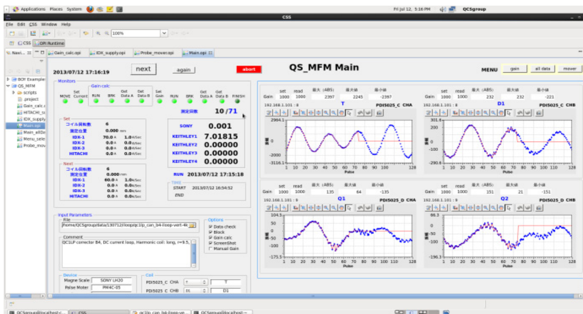
Figure 3: Control screen for the superconducting magnetic field measurement system.
