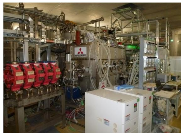
Figure 2: Injector cryomodule at the beam line.
