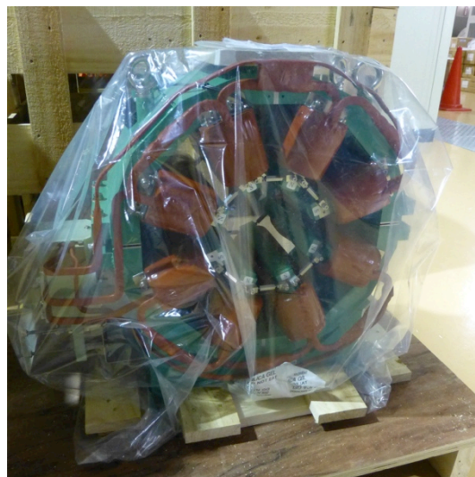
Figure 1: Octupole Magnet delivered to J-PARC MR.
