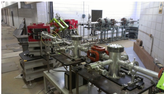
Figure 3: Replaced dispersion section omitting straight beam line to a synchrotron.
