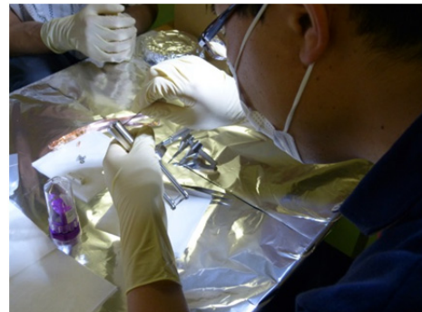
Figure 5: Replacing a cathode of injector linac.
