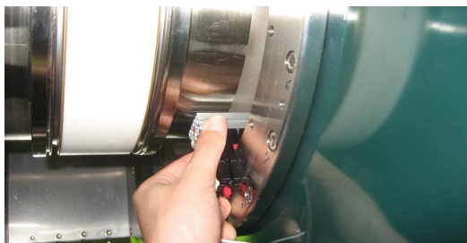
Figure 1: Finemet yoke sensor inserted between beam pipe and cavity tank for buckling check.
