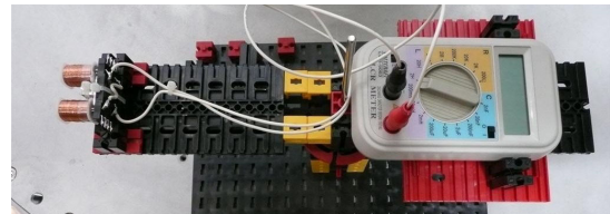
Figure 8: Buckling detection test with relay sensor.
