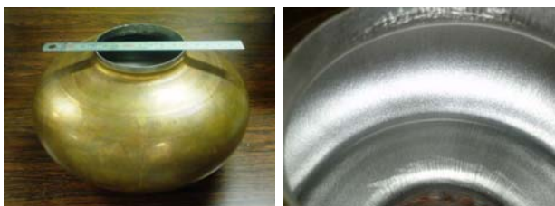
Fig. 9. Seamless cavity (Nb/Cu clad) left: inside of the cavity
