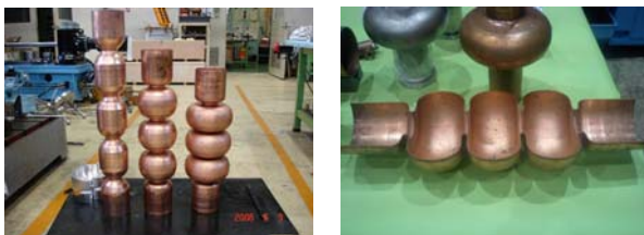
Fig. 1. Seamless three-cell cavities made by necking and hydroforming (test modules made of copper).
