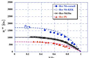
Figure 2: Data fitting by the proposed formula (2) on Nb, Nb<sub>3</sub>Sn, and Pb cavities.
