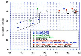
Figure 1: History of high gradient with an L-band single cell cavity.
