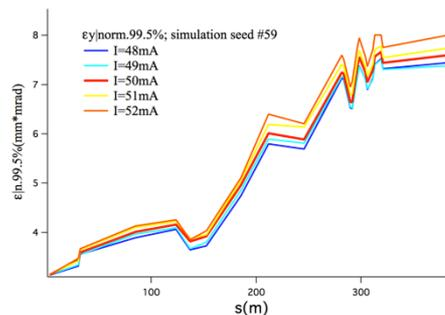
Figure 10: Simulated horizontal 99.5% emittance for error seed #59.
