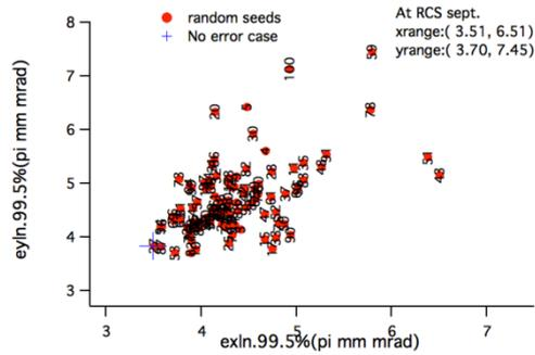
Figure 5: Simulated output transverse emittance with errors for the baseline design of the J-PARC linac.
