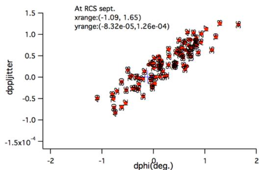
Figure 7: Simulated energy and phase jitter of output beam with errors for the baseline design of the J-PARC linac, with the 2-debuncher system.
