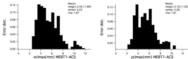
Figure 8: Simulated beam maximum orbit distortion, without correction, from MEBT1 to end of ACS.
