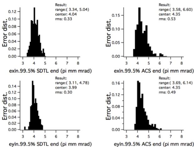
Figure 3: Statistical results of simulated transverse emittance at entry and exit of new ACS part with errors for the baseline design of the J-PARC linac upgrade.
