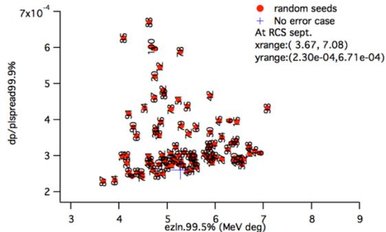
Figure 6: Simulated output longitudinal emittance with errors for the baseline design of the J-PARC linac.
