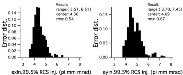
Figure 4: Statistical results of simulated output transverse emittance with errors for the baseline design of the J-PARC linac upgrade.
