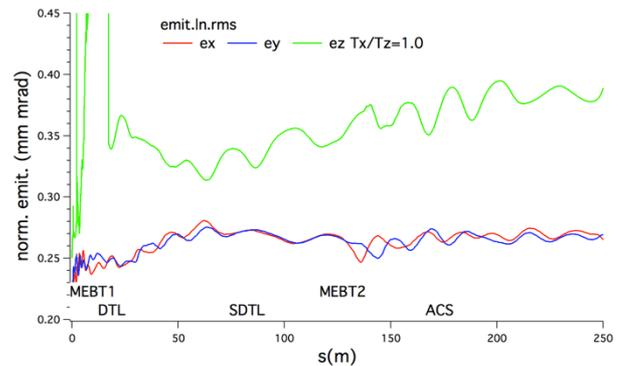
Figure 2: Simulated rms emittance for the baseline design of the J-PARC linac .
