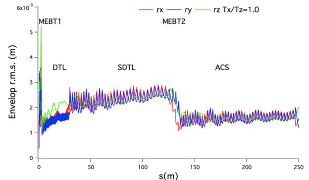
Figure 1: Simulated rms envelope for the baseline design of the J-PARC linac .
