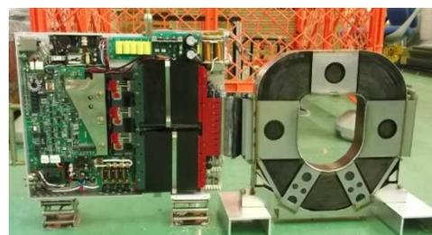
Figure 3: IGBT and an induction core.
