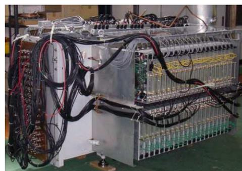
Figure 2: Induction accelerator modules.
