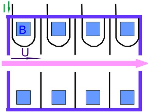
Figure 4: Induction accelerator composed of four individual modules placed in series.
