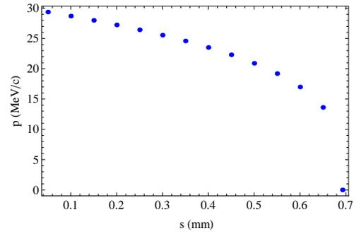
Figure 6: Energy moderation of muons in terms of momentum as a function of degrader thickness.
