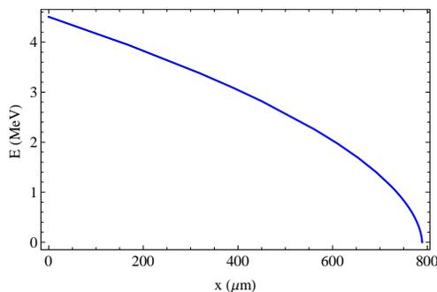
Figure 5: Energy moderation of muons as a function of degrader thickness.
