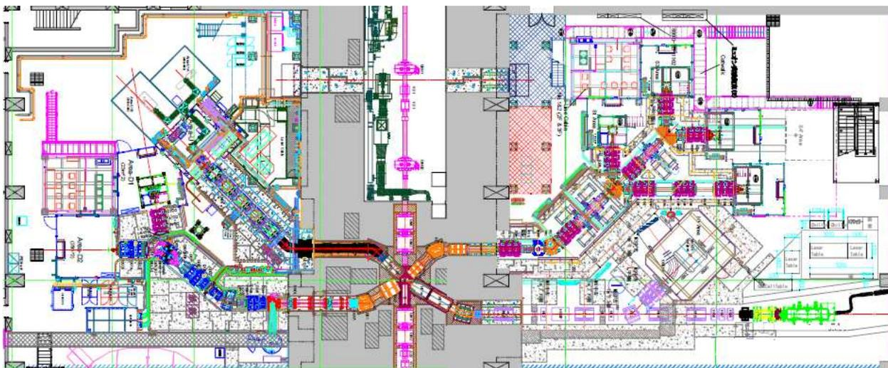
Figure 1: Top view of the muon production target and associated four beam transport lines (J-PARC MLF). Two of these beam lines are extracted at the angle of 60 degrees to the proton beam line (backward), and the others are at 135 degrees (forward).
