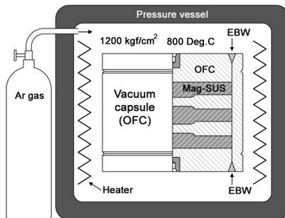
Fig. 6: HIP diffusion bonding process.
