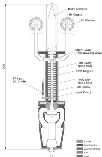
Fig. 1: Cut away view of the first C-band (5712 MHz) 50 MW-class PPM type klystrons (TOSHIBA E3747).
