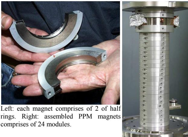
Fig. 2: PPM magnet mounted on the main body of klystron.
