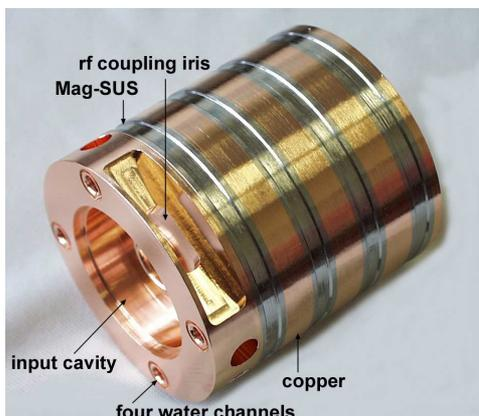
Fig. 7: The diffusion bonded PPM modules, after machining an input rf-cavity, an iris, the beam hole and four water channels.
