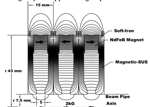
Fig. 3: Cutaway view of the PPM structure and the magnetic-field pattern.
