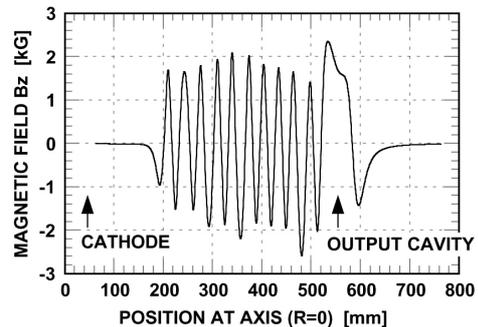
Fig. 4: Measured field profile along the axis at the center. ( $B_z, r=0$ )
