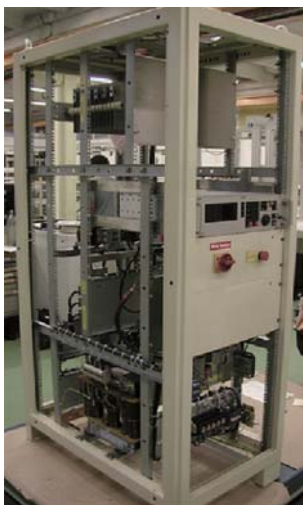
PSU for Superconducting magnets up to 5000 A, up to ± 60 V
