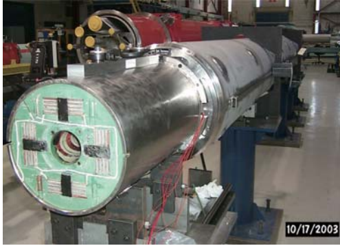
LHC (Geneva – SWITZERLAND) 33 superconducting X-Y corrector dipoles
